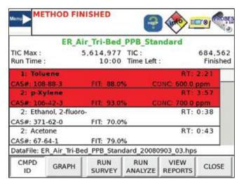
The highlighted chemicals are linked to the on-board NIOSH database for actionable information that can be used to quickly assess danger level.
