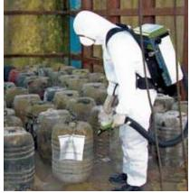
HAPSITE ER has the capability to identify analytes in the PPM(parts per million) – PPT(parts per trillion) range. The GC column provides sharp chromatography and excellent resolution. During the quantitation method, the front panel clearly displays what chemicals are present, their concentration, and access to information regarding the degree of danger — to help make quick decisions affecting life, health and safety.
